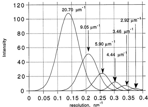
**FIG. 3.** Plot of the coherent component for each reciprocal defocus in the 3DFFT of the through focus series used to restore Fig. 1A.
