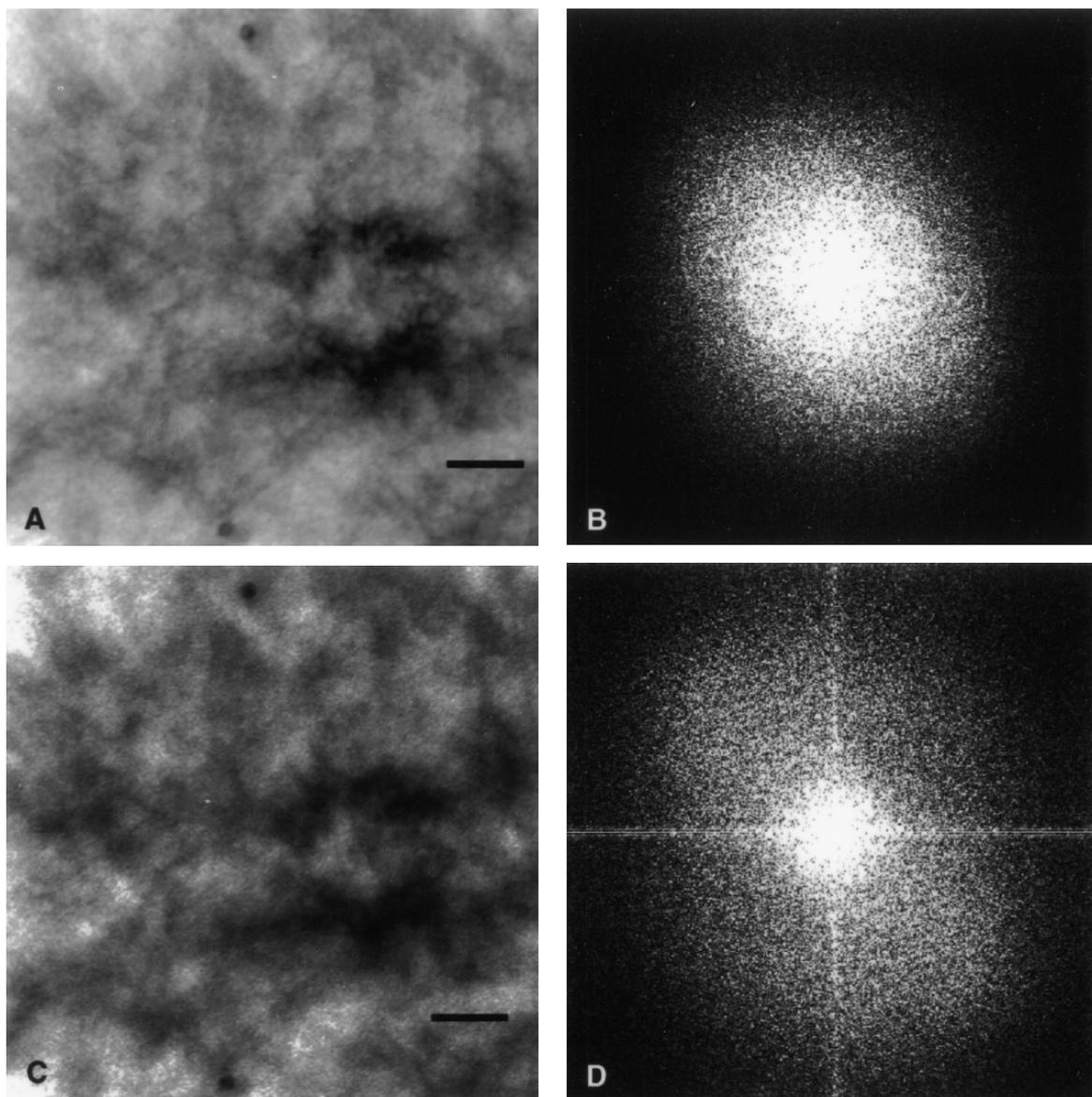
**FIG. 1.** Exit wavefront restoration (A) from 40 through focus images and its diffractogram (B); 905-nm defocused image (C) and its diffractogram (D). Scale bar, 100 nm, resolution limit is  $(2.41 \text{ nm})^{-1}$ .
