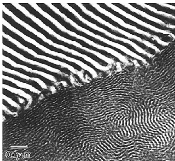
Figure 2. Transmission electron micrograph of an equimolar SI/(SI) 4 blend, revealing that the blend is immiscible and that the SI and (SI) 4 phases (large and small lamellae, respectively) are separated by relatively sharp interfaces.
